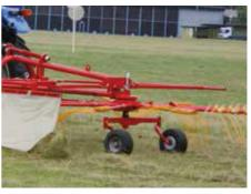
Swivel wheel suspension facilitates rake operation in narrow U-turns.
