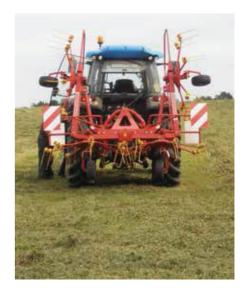
**Transport position** external rotors are folded to the transport position by the hydraulic system.
