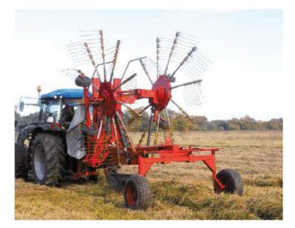
The rotors are set in transport position by the hydraulic system.
