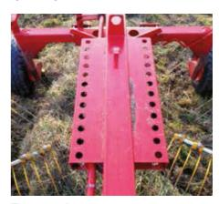
**Transport bar** during trips to longer distances, the raking arms can be securely installed in the holes of the middle transport bar.
