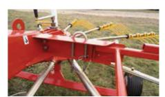
Rotor interlock allows disassembly of only side arms for transport.
