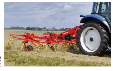
Angle of spread 4-step adjustment of the angle of spread allows setting grass processing intensity according to the needs.
