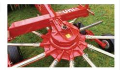
Adjusting of tines is easy controlled directly on the gearbox with a special wheel lock.
